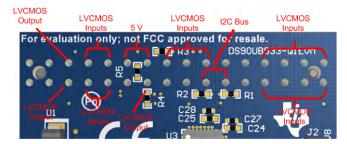
Figure 2-3. Parallel Input Connector on Serializer Board
