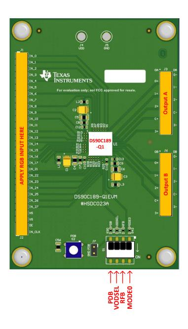
Figure 2. Demo Board Connections
