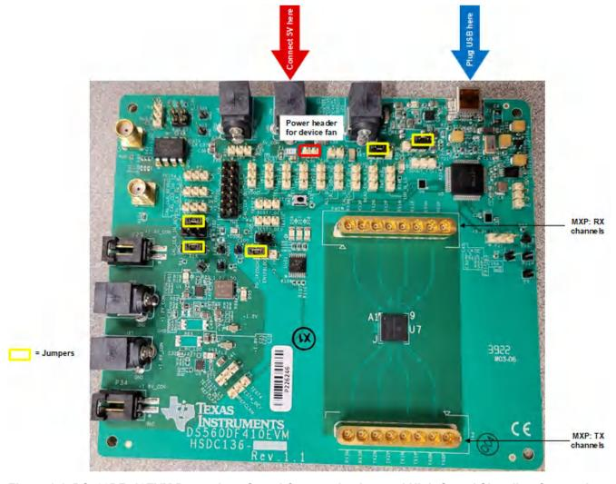
Figure 1-1. DS560DF410EVM Power, Low-Speed Communication, and High-Speed Signaling Connections
