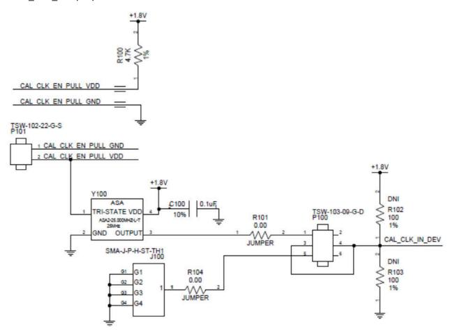
Figure 1-3. DS560DF410EVM Schematic Portion for CAL\_CLK\_IN Input Circuit
