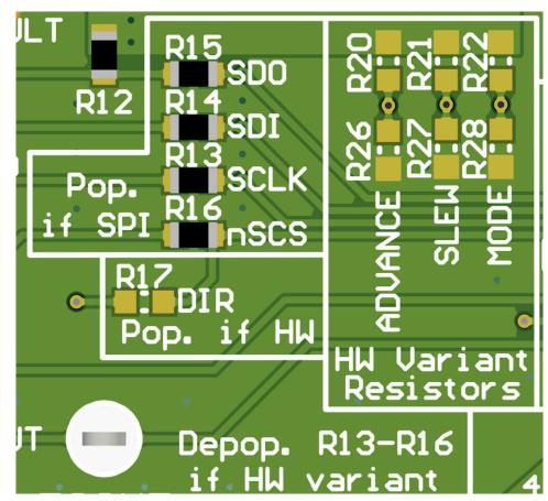
Figure 2-8. Resistors for MCT8315ZR (SPI variant)
