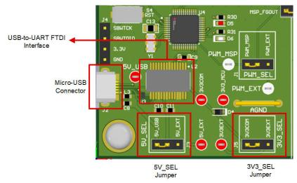
Figure 2-4. Micro-USB Connector and UART for MCT8315ZEVM
