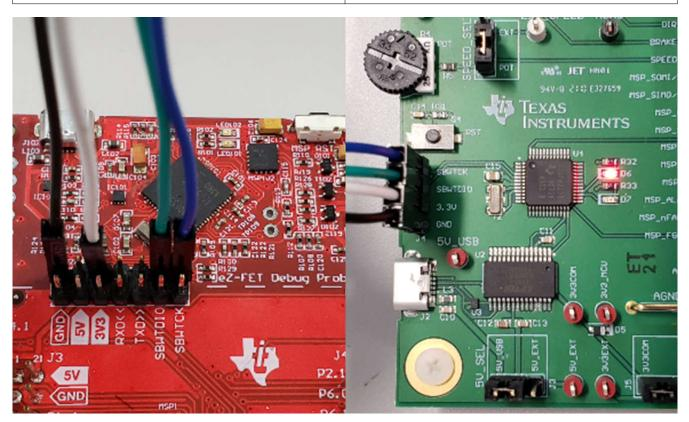
Figure 3-4. MSP430 LaunchPad<sup>™</sup> eZ-FET Probe Connected to MCT8315ZEVM
