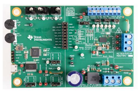
MCT8315ZEVM Printed Circuit Board (PCB - Top View)
