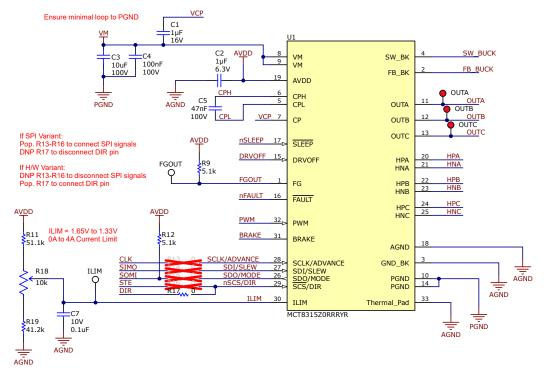
Figure 4-1. MCT8315Z 3-Phase Sensored Trapezoidal Motor Driver Schematic
