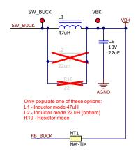
Figure 4-3. Buck Regulator Schematic
