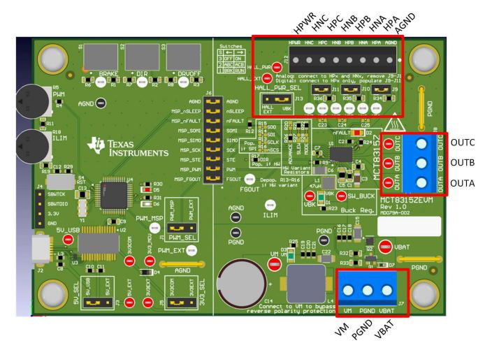
Figure 2-3. Connections from Motor to MCT8315ZEVM
