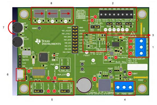
Figure 2-1. Reference for Quick Start Guide
