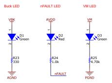
Figure 4-7. Status LEDs Schematic
