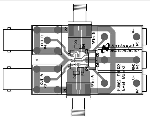
Figure 7. Layout for LMV862, All Layers
