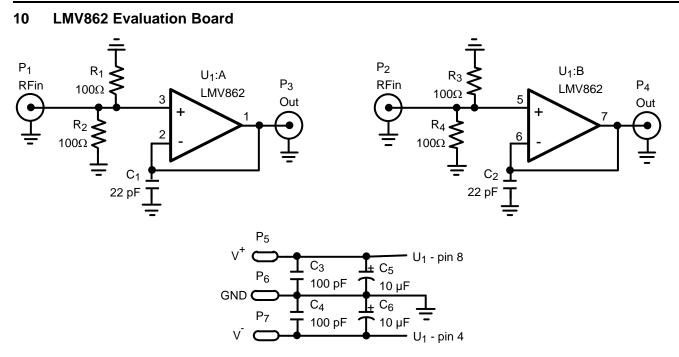
Figure 6. Schematic for LMV862, Coupling RF Signal to the IN+ Pin
