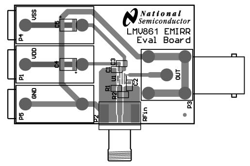
Figure 4. Layout for LMV861, All Layers
