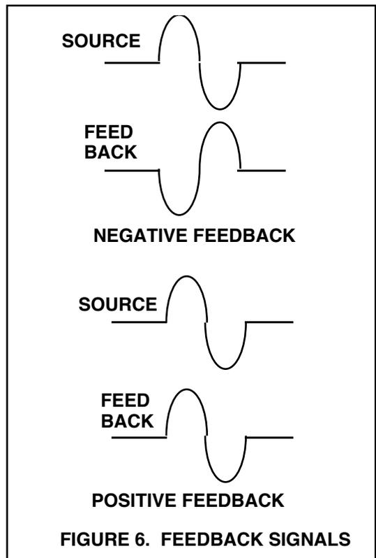
Positive feedback occurs when the feedback signal has the same polarity as the source signal. In this case, the loop responds in the same direction as any change which occurs at the output. This is clearly unstable, since it does not cancel out changes in output voltage, but amplifies them.
