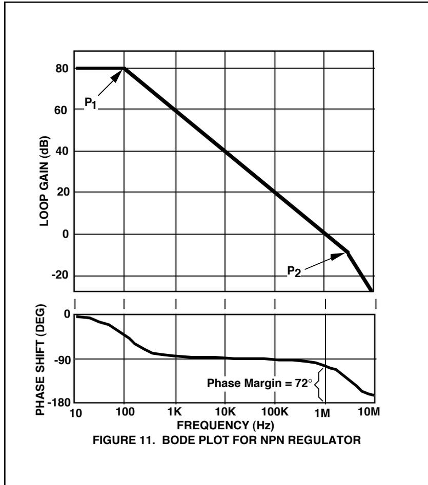
FIGURE 11. BODE PLOT FOR NPN REGULATOR
