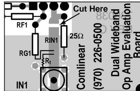
Figure 2: Modifications for Inverting Gains (CLC730038 board shown)
