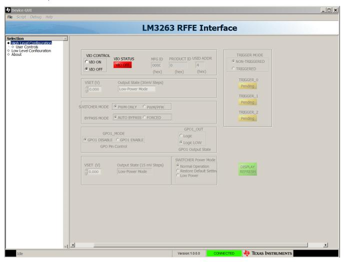
Figure 7. LM3263 GUI Initial Screen
