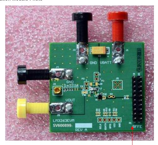
20 pin Connector (VIO, SCLK, SDATA, GND connect to LM8335EVM.)
