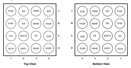
Figure 5. Connection Diagram
