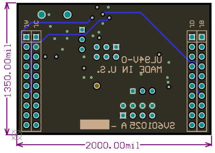
Figure 4-5. Bottom Layer Routing
