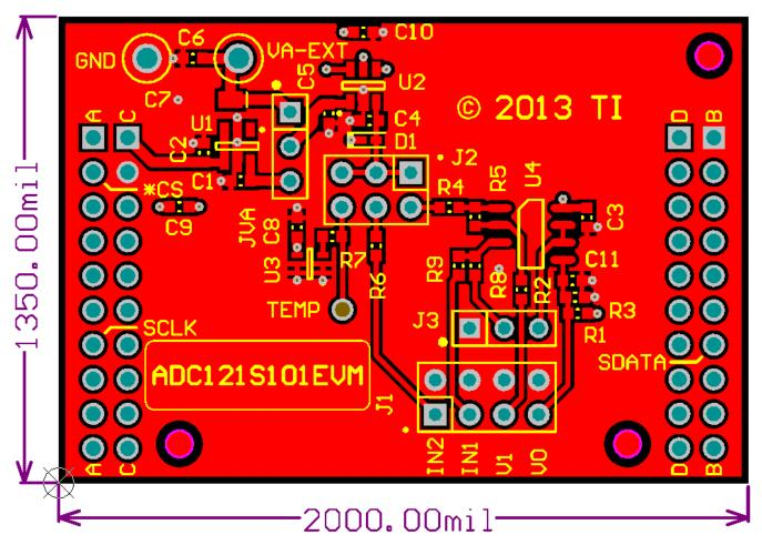
Figure 4-1. Top Assembly Layer
