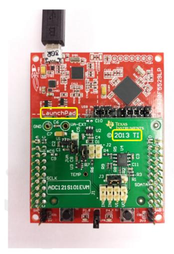
Figure 3-1. ADC121S101EVM Attached to MSP430
