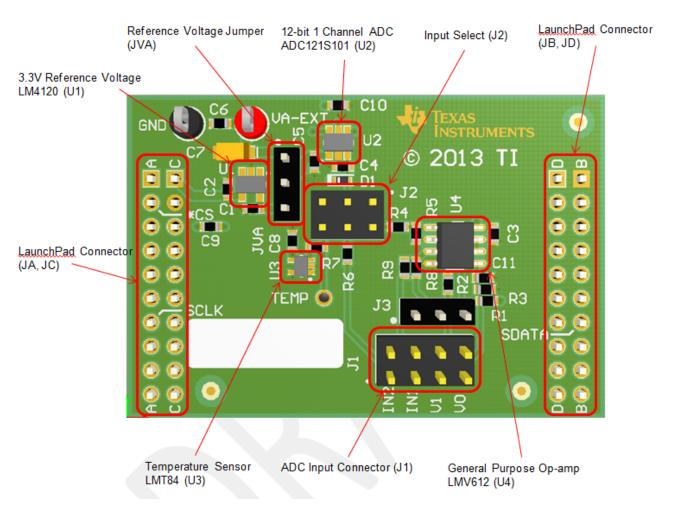
Figure 1-1. ADC121S101EVM Evaluation Board
