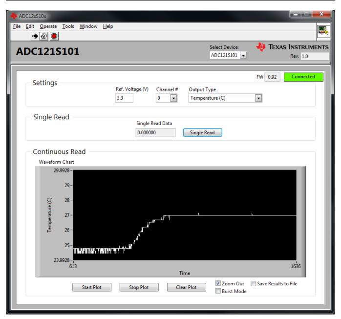
Figure 3-4. Testing the Part
