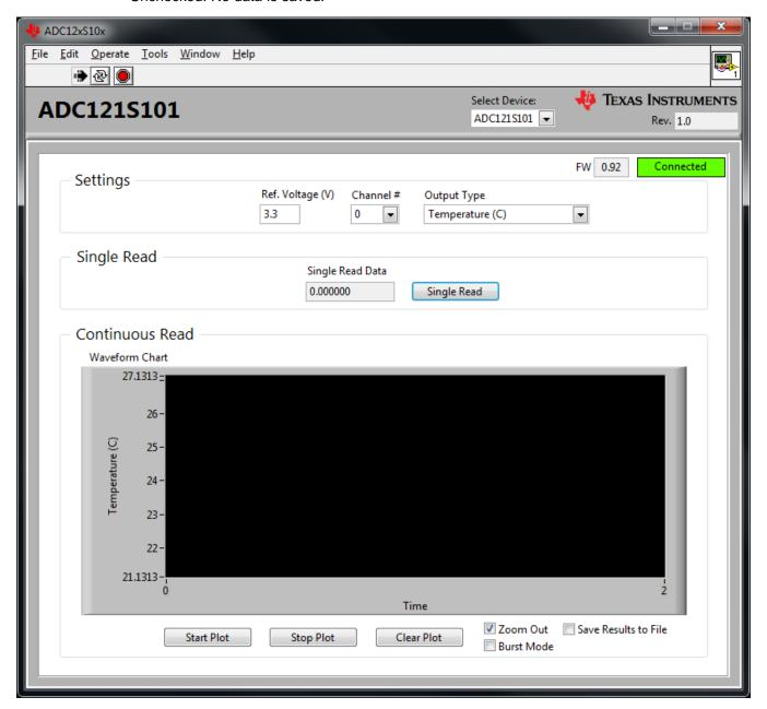
Figure 3-3. Selectable Fields in GUI
