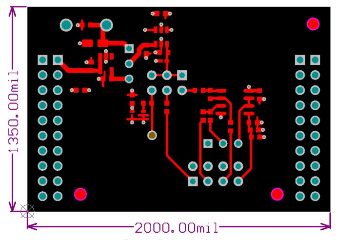
Figure 4-2. Top Layer Routing
