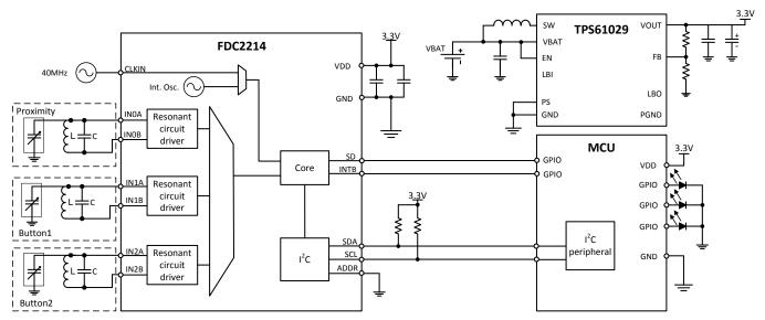
Figure 2. System Level Block Diagram
