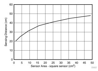
Figure 4. Sensor Size Area Versus Sensing Distance
