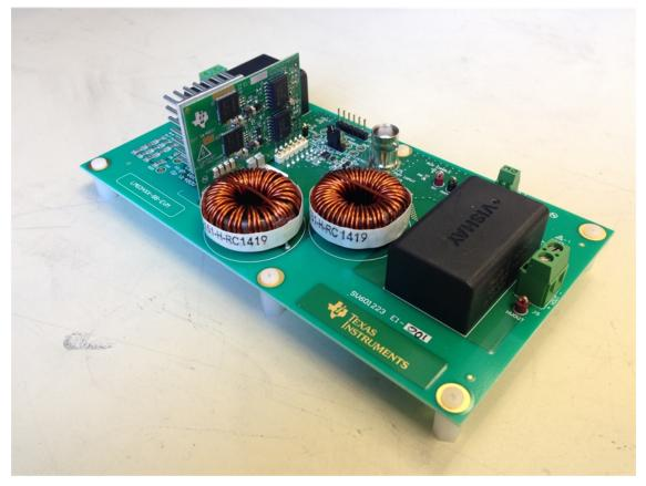
Figure 6. LMG3410-HB-EVM Connected with LMG34XX-BB-EVM
