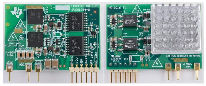
Figure 2. Front and Back Side Photos of LMG3410-HB-EVM
