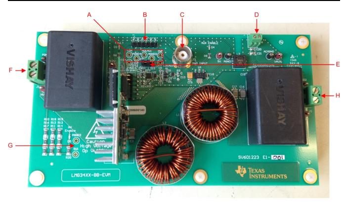
Figure 7. Recommended Connection Points
