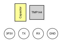
Figure 2. TMP144EVM Pin Connections
