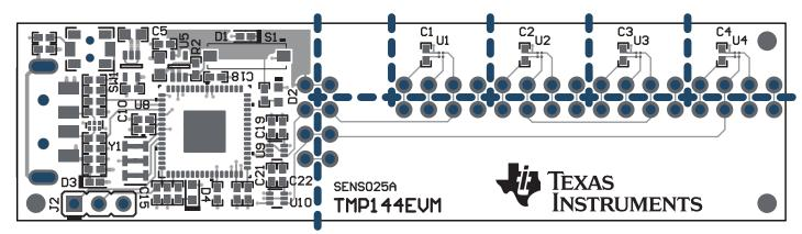
Figure 9. Printed-Circuit Board
