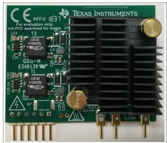
Figure 2. Top Side View of LMG341xEVM-018
