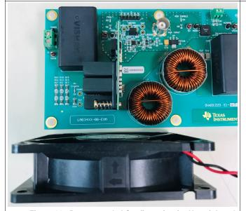
Figure 11. Recommended Configuration for Heatsink and Fan
