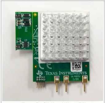
Figure 2. Top Side View of LMG3411EVM-031
