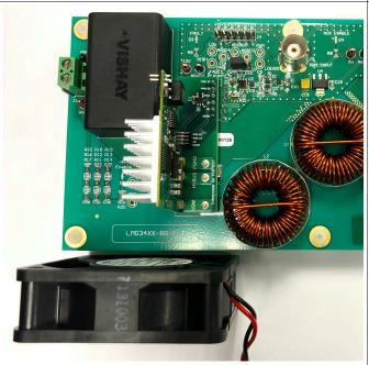
Figure 13. Recommended Configuration for Heatsink and Fan
