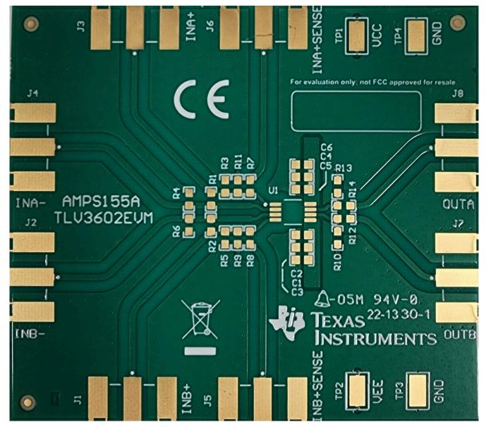
Figure 1-1. TLV3602EVM Board Top View
