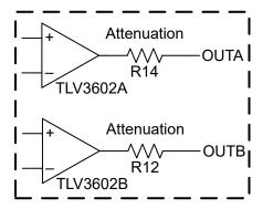
Figure 5-4. Output Side Block Diagram
