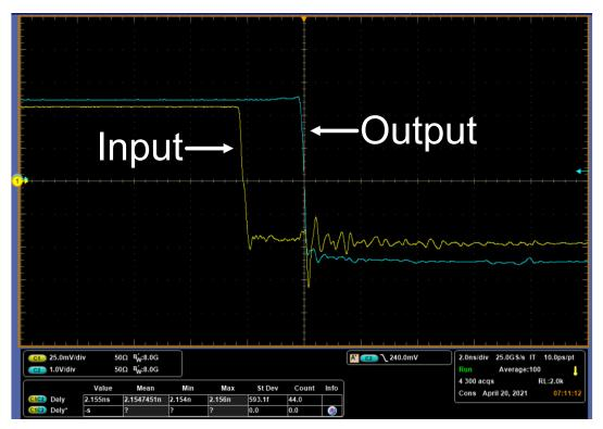
Figure 4-3. Propagation Delay Fall Portion
