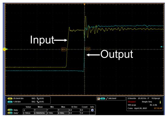
Figure 4-2. Propagation Delay Rise Portion
