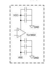
Figure 5-2. TLV3602EVM Supply Voltage Schematic
