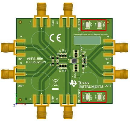
Figure 5-1. TLV3602EVM Supply Voltage Connection
