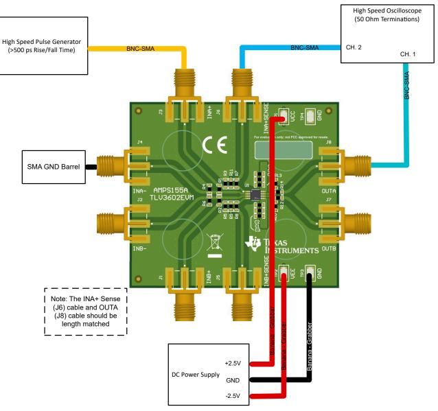
Figure 4-1. TLV3602EVM Quick Start Setup
