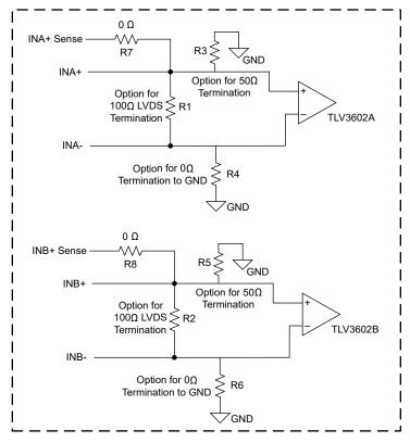
Figure 5-3. Input Side Schematic
