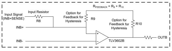
Figure 5-6. TLV3602 Hysteresis Schematic for Channel B
