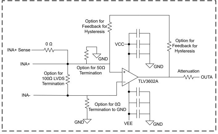
Figure 2-1. Block Diagram Per Channel
