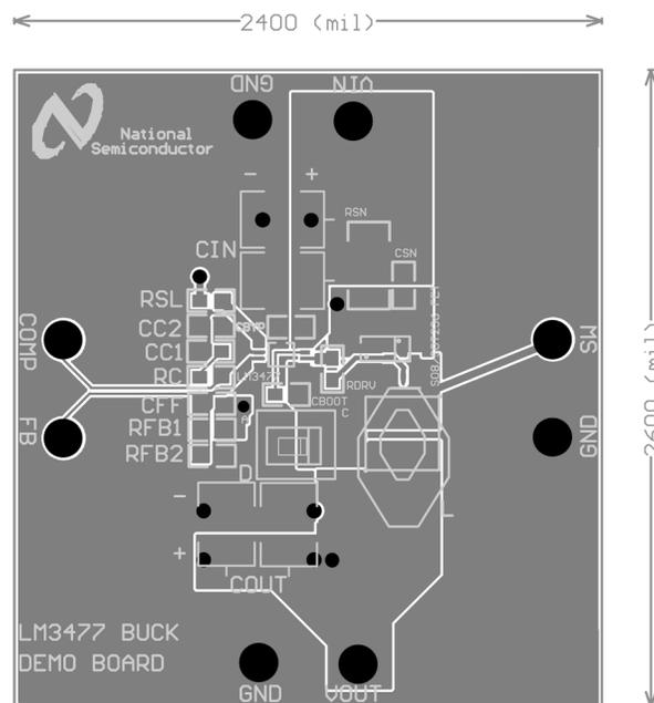
**Figure 7. LM3477 Evaluation Board PCB Layout (Top Side)**
