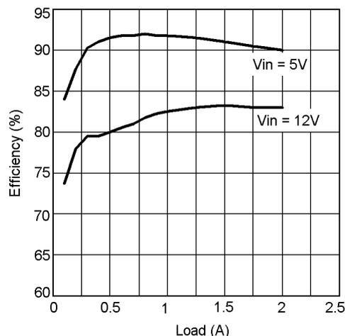
**Figure 2. Efficiency vs Load V<sub>OUT</sub> = 3.3 V**
