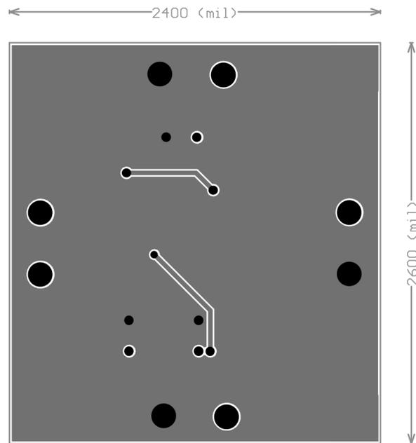
**Figure 8. LM3477 Evaluation Board PCB Layout (Bottom Side)**
