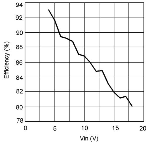
**Figure 3. Efficiency vs  $V_{IN}$**
