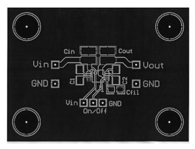
Figure 2. Typical Layout, Top View (magnification 1.5X)
