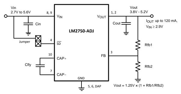
Figure 1. Evaluation Board Schematic
