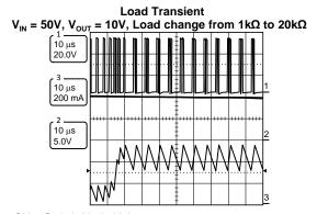
CH1: Switch Node Voltage CH2: Output Voltage CH3: Inductor Current
