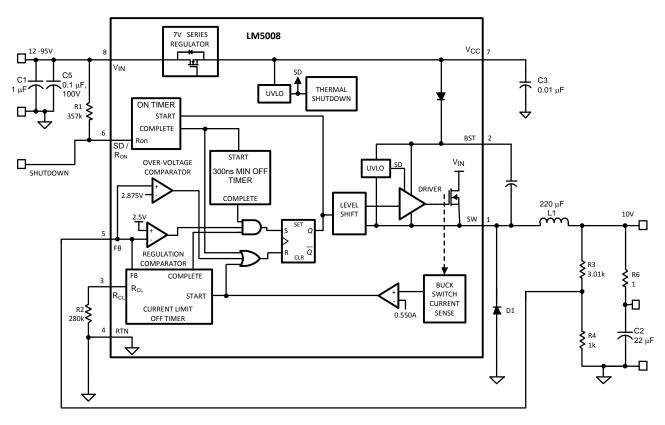
Figure 2. Evaluation Board Schematic Diagram
