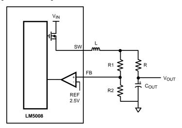
Figure 1. Low Ripple Configuration Output
