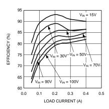
Figure 3. LM5008 Efficiency
