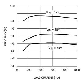
Figure 2. Efficiency vs Load Current
