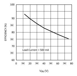
Figure 3. Efficiency vs V<sub>IN</sub>
