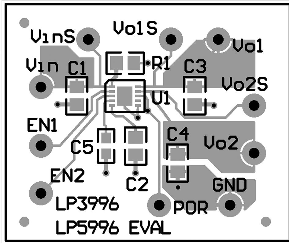
Figure 2. Evaluation Board Component and Pin Layout
