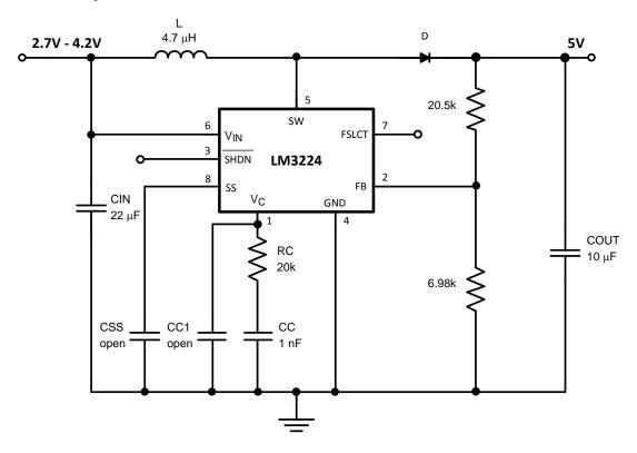
Figure 1. Schematic
