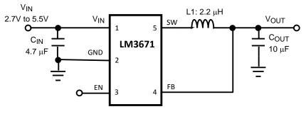
Figure 1. Fixed Output Voltage — Typical Application Circuit
