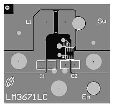
Figure 9. Top Layer (6-pin USON)
