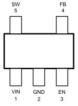
Figure 3. SOT23–5, Top View
