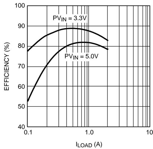
Figure 3. LM2852X Typical Efficiency for 2.5 V Output
