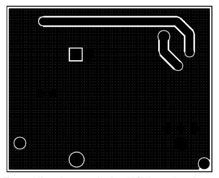
Figure 4. LM3489 Demonstration Board PCB Bottom Layer Layout
