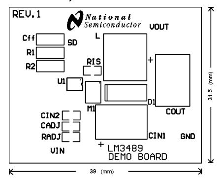
Figure 2. LM3489 Demonstration Board PCB Top Overlay
