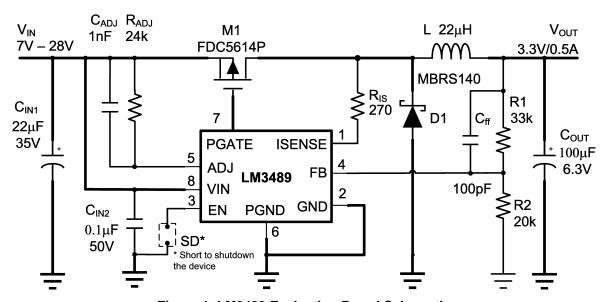
Figure 1. LM3489 Evaluation Board Schematic
