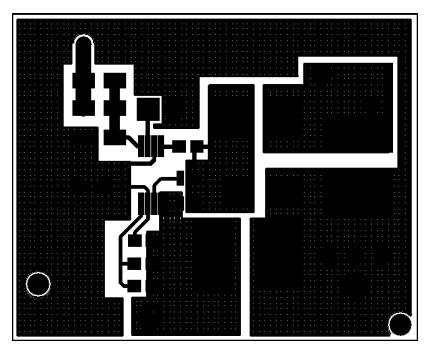
Figure 3. LM3489 Demonstration Board PCB Top Layer Layout
