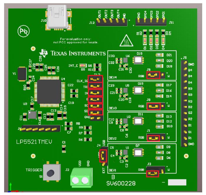
Figure 1. Evaluation Board Connectors and Setup
