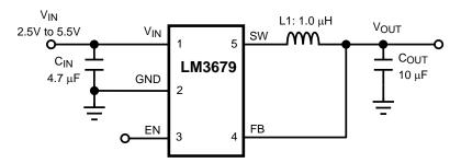
Figure 1. Typical Application Circuit
