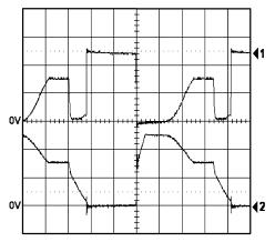
Horizontal Resolution: 0.5 µs/div Trace 1: The HO pin voltage. 20V/div Trace 2: The LO pin voltage. 20V/div
