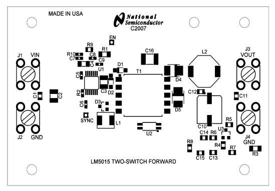
Figure 1. Evaluation Board Layout
