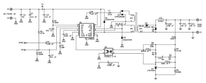
Figure 6. Schematic of Isolated Two-Switch Flyback DC-DC Regulator Configuration
