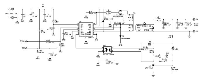
Figure 2. Schematic of Isolated Two Forward DC-DC Regulator (Factory Default)
