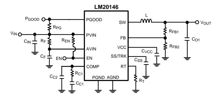
Figure 1. Evaluation Board Schematic
