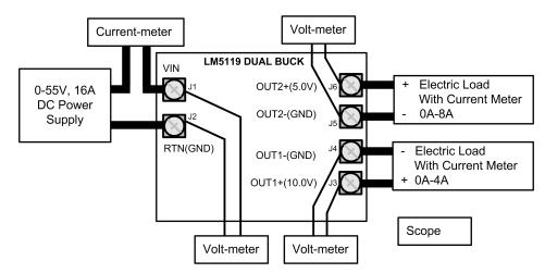
Figure 1. Typical Evaluation Setup
