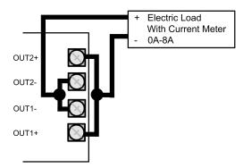
Figure 8. Load Connection for Single Output
