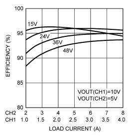
Figure 7. Typical Efficiency vs Load Current
