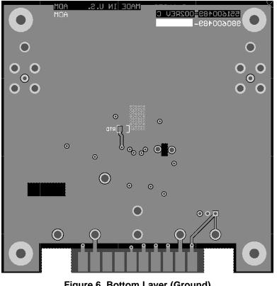
Figure 6. Bottom Layer (Ground) Heat Sinking Layer
