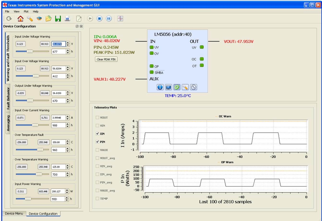
Figure 6. LM5056 GUI with Telemetry Plotting Tool Enabled
