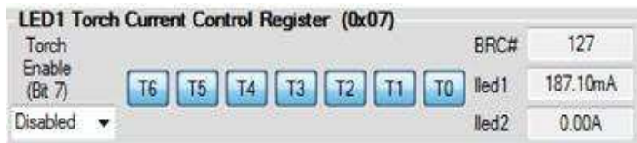
Figure 22. LED1 Torch Current Control Register
