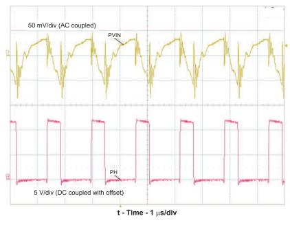
Figure 11. LMZ31506EVM-692 Input Voltage Ripple
