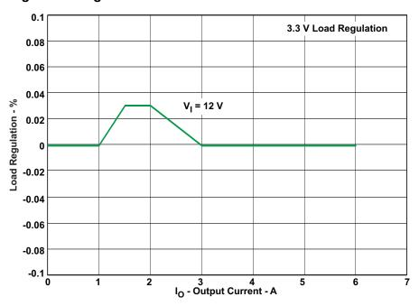
Figure 6. Load Regulation at 25°C
