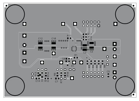
Figure 16. LMZ3150xEVM-692 Bottom-Side Layer and Assembly
