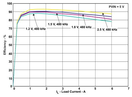
Figure 5. Efficiency vs Output Voltage/Frequency at 25°C
