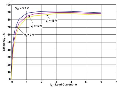
Figure 2. Efficiency vs Voltage at 25°C
