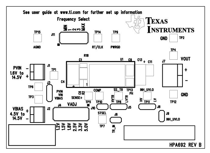
Figure 13. LMZ3150xEVM-692 Top-Side Layer and Assembly
