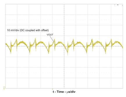
Figure 10. LMZ31506EVM-692 Output Voltage Ripple
