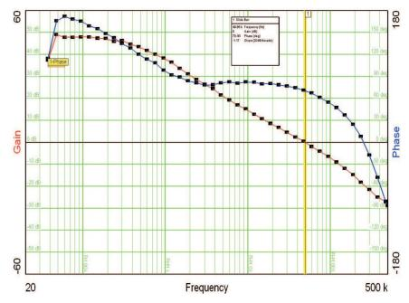
Figure 9. LMZ31506EVM-692 Loop Response at 25°C
