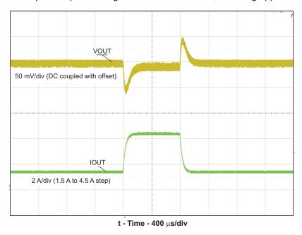
Figure 8. 3.3-V LMZ31506HEVM-692 Transient Response at 25°C
