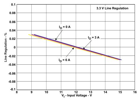
Figure 7. Line Regulation at 25°C
