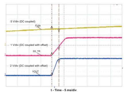
Figure 12. LMZ31506EVM-692 Start-Up Waveforms With Rising PVIN
