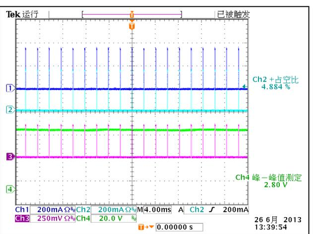
115Vac PWM Dimming 5% Ch1:LED4 Ch2:LED5 CH3:LED6 CH4:Vout
