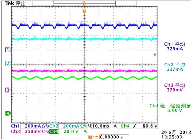
115Vac Full load ripple Ch1:LED1 Ch2:LED2 CH3:LED3 CH4:Vout
