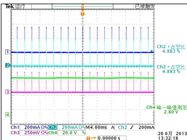
115Vac PWM Dimming 5% Ch1:LED1 Ch2:LED2 CH3:LED3 CH4:Vout
