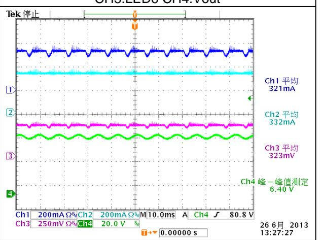
230Vac Full load ripple Ch1:LED4 Ch2:LED5 CH3:LED6 CH4:Vout
