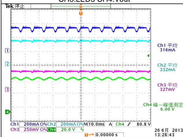
230Vac Full load ripple Ch1:LED1 Ch2:LED2 CH3:LED3 CH4:Vout
