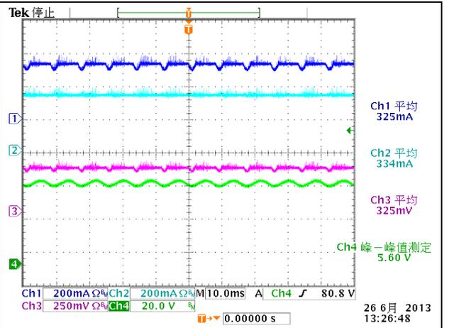
115Vac Full load ripple Ch1:LED4 Ch2:LED5 CH3:LED6 CH4:Vout
