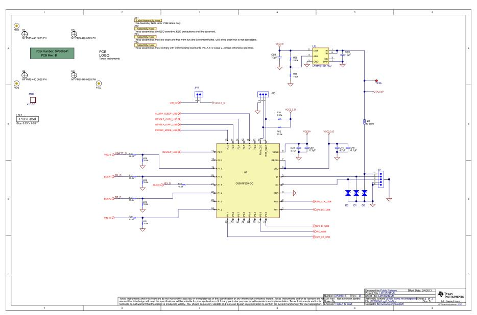
Figure 6. LM10524EVM Schematic
