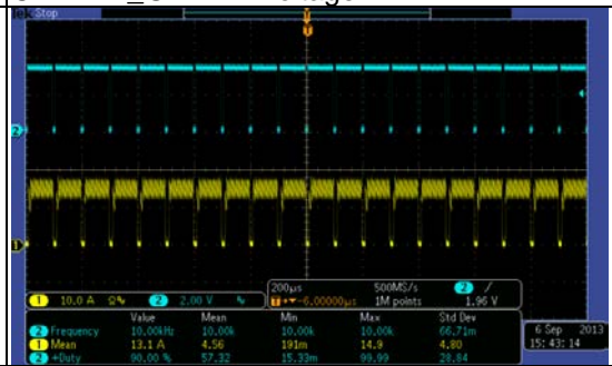
90% Dimming CH1: Blue LED current CH2: EN_BLUE Voltage
