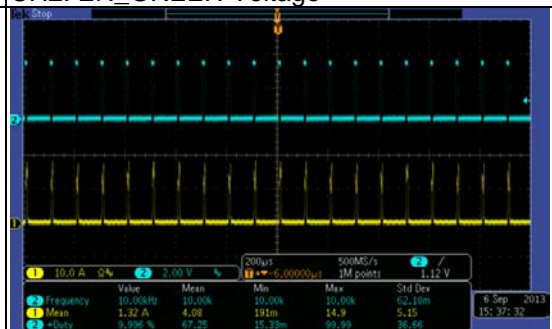
10% Dimming CH1: Blue LED current CH2: EN_BLUE Voltage
