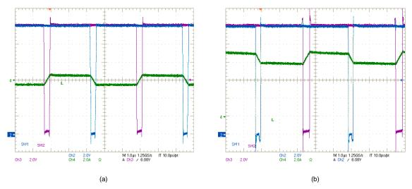
Figure 12. SW1, SW2,  $I_L$  Waveforms:  $V_{IN} = 12 \text{ V}$ ,  $V_{OUT} = 12 \text{ V}$ , (a)  $I_{OUT} = 0 \text{ A}$ , (b)  $I_{OUT} = 6 \text{ A}$
