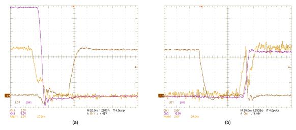
Figure 31. SW1, LO1, (HO1–SW1) Voltages:  $V_{IN}$  = 36 V,  $V_{OUT}$  = 12 V,  $I_{OUT}$  = 6 A, (a) OFF, (b) ON
