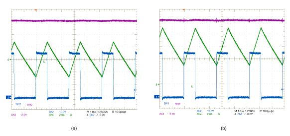
Figure 17. SW1, SW2,  $I_L$  Waveforms:  $V_{IN}$  = 36 V,  $V_{OUT}$  = 12 V, (a)  $I_{OUT}$  = 0 A, (b)  $I_{OUT}$  = 6 A
