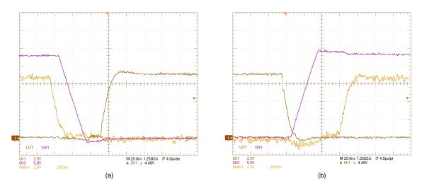
Figure 23. SW1, LO1, (HO1–SW1) Voltages:  $V_{IN}$  = 24 V,  $V_{OUT}$  = 12 V,  $I_{OUT}$  = 0 A, (a) OFF, (b) ON
