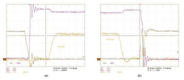
Figure 39. SW2, LO2, (HO2–SW2) Voltages:  $V_{IN} = 8 \text{ V}$ ,  $V_{OUT} = 12 \text{ V}$ ,  $I_{OUT} = 6 \text{ A}$ , (a) OFF, (b) ON
