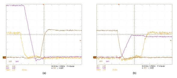
Figure 21. SW1, LO1, (HO1–SW1) Voltages:  $V_{IN} = 14 \text{ V}$ ,  $V_{OUT} = 12 \text{ V}$ ,  $I_{OUT} = 0 \text{ A}$ , (a) OFF, (b) ON
