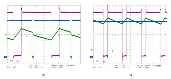
Figure 11. SW1, SW2,  $I_L$  Waveforms:  $V_{IN} = 10 \text{ V}$ ,  $V_{OUT} = 12 \text{ V}$ , (a)  $I_{OUT} = 0 \text{ A}$ , (b)  $I_{OUT} = 6 \text{ A}$
