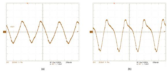
Figure 49.  $V_{OUT}$  ripple:  $V_{IN} = 36 \text{ V}$ ,  $V_{OUT} = 12 \text{ V}$ , (a)  $I_{OUT} = 0 \text{ A}$ , (b)  $I_{OUT} = 6 \text{ A}$
