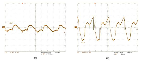
Figure 44.  $V_{OUT}$  ripple:  $V_{IN} = 8 \text{ V}$ ,  $V_{OUT} = 12 \text{ V}$ , (a)  $I_{OUT} = 0 \text{ A}$ , (b)  $I_{OUT} = 6 \text{ A}$
