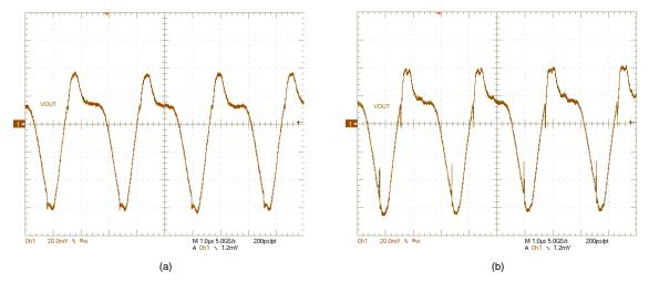
Figure 50.  $V_{OUT}$  ripple:  $V_{IN}$  = 42 V,  $V_{OUT}$  = 12 V, (a)  $I_{OUT}$  = 0 A, (b)  $I_{OUT}$  = 6 A
