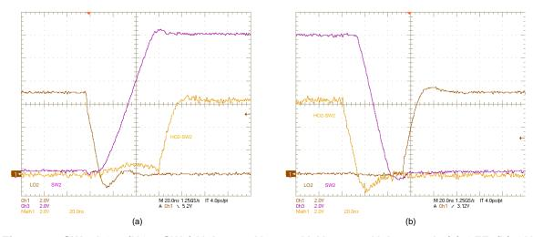
Figure 37. SW2, LO2, (HO2–SW2) Voltages:  $V_{IN} = 14 \text{ V}$ ,  $V_{OUT} = 12 \text{ V}$ ,  $I_{OUT} = 0 \text{ A}$ , (a) OFF, (b) ON
