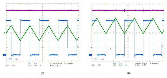
Figure 16. SW1, SW2,  $I_L$  Waveforms:  $V_{IN}$  = 24 V,  $V_{OUT}$  = 12 V, (a)  $I_{OUT}$  = 0 A, (b)  $I_{OUT}$  = 6 A
