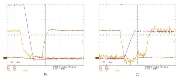
Figure 24. SW1, LO1, (HO1–SW1) Voltages:  $V_{IN}$  = 36 V,  $V_{OUT}$  = 12 V,  $I_{OUT}$  = 0 A, (a) OFF, (b) ON
