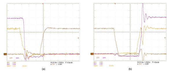
Figure 26. SW1, LO1, (HO1–SW1) Voltages:  $V_{IN} = 10.5 \text{ V}$ ,  $V_{OUT} = 12 \text{ V}$ ,  $I_{OUT} = 6 \text{ A}$ , (a) OFF, (b) ON
