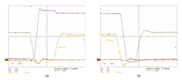
Figure 35. SW2, LO2, (HO2–SW2) Voltages:  $V_{IN}$  = 10 V,  $V_{OUT}$  = 12 V,  $I_{OUT}$  = 0 A, (a) OFF, (b) ON
