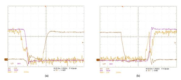
Figure 32. SW1, LO1, (HO1–SW1) Voltages:  $V_{IN}$  = 42 V,  $V_{OUT}$  = 12 V,  $I_{OUT}$  = 6 A, (a) OFF, (b) ON
