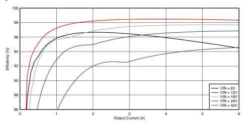
Figure 5. Efficiency vs. Output Current
