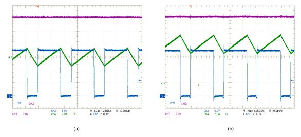
Figure 15. SW1, SW2,  $I_L$  Waveforms:  $V_{IN}$  = 18 V,  $V_{OUT}$  = 12 V, (a)  $I_{OUT}$  = 0 A, (b)  $I_{OUT}$  = 6 A
