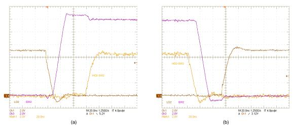
Figure 33. SW2, LO2, (HO2–SW2) Voltages:  $V_{IN} = 6 \text{ V}$ ,  $V_{OUT} = 12 \text{ V}$ ,  $I_{OUT} = 0 \text{ A}$ , (a) OFF, (b) ON
