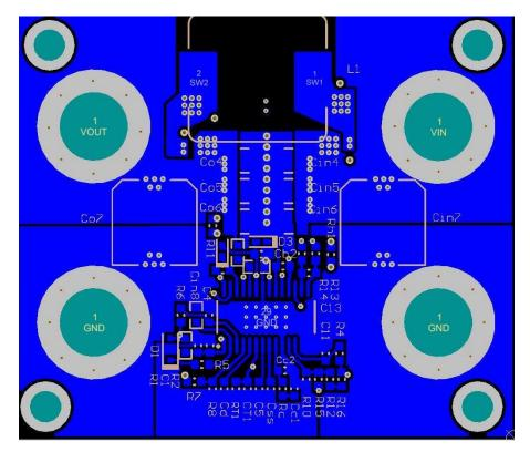
Figure 57. Bottom Copper (Bottom view)
