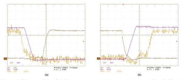
Figure 25. SW1, LO1, (HO1–SW1) Voltages:  $V_{IN}$  = 42 V,  $V_{OUT}$  = 12 V,  $I_{OUT}$  = 0 A, (a) OFF, (b) ON
