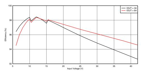
Figure 6. Efficiency vs. Input Voltage
