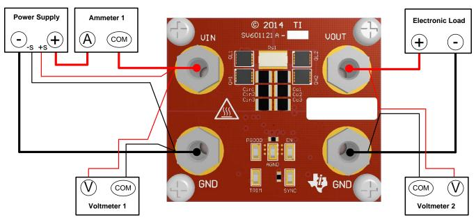
Figure 4. Test Setup Connection Diagram
