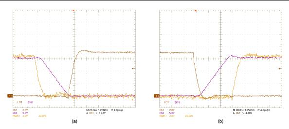
Figure 22. SW1, LO1, (HO1–SW1) Voltages:  $V_{IN}$  = 16 V,  $V_{OUT}$  = 12 V,  $I_{OUT}$  = 0 A, (a) OFF, (b) ON
