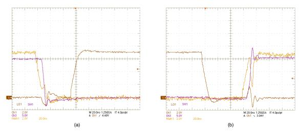
Figure 29. SW1, LO1, (HO1–SW1) Voltages:  $V_{IN}$  = 16 V,  $V_{OUT}$  = 12 V,  $I_{OUT}$  = 6 A, (a) OFF, (b) ON
