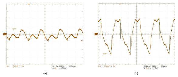
Figure 43.  $V_{OUT}$  ripple:  $V_{IN} = 6 \text{ V}$ ,  $V_{OUT} = 12 \text{ V}$ , (a)  $I_{OUT} = 0 \text{ A}$ , (b)  $I_{OUT} = 6 \text{ A}$
