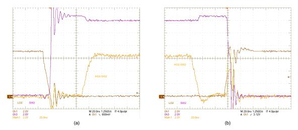
Figure 38. SW2, LO2, (HO2–SW2) Voltages:  $V_{IN}$  = 6 V,  $V_{OUT}$  = 12 V,  $I_{OUT}$  = 6 A, (a) OFF, (b) ON
