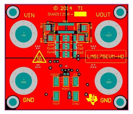
Figure 52. Top Copper (Top view)
