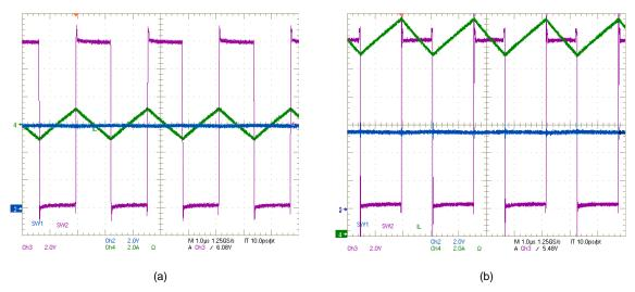
Figure 9. SW1, SW2,  $I_L$  Waveforms:  $V_{IN}$  = 6 V,  $V_{OUT}$  = 12 V, (a)  $I_{OUT}$  = 0 A, (b)  $I_{OUT}$  = 6 A
