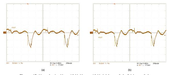
Figure 45.  $V_{OUT}$  ripple:  $V_{IN}$  = 12 V,  $V_{OUT}$  = 12 V, (a)  $I_{OUT}$  = 0 A, (b)  $I_{OUT}$  = 6 A
