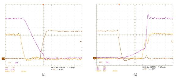
Figure 19. SW1, LO1, (HO1–SW1) Voltages:  $V_{IN} = 10.5 \text{ V}$ ,  $V_{OUT} = 12 \text{ V}$ ,  $I_{OUT} = 0 \text{ A}$ , (a) OFF, (b) ON
