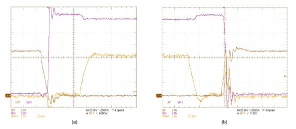
Figure 42. SW2, LO2, (HO2–SW2) Voltages:  $V_{IN}$  = 14 V,  $V_{OUT}$  = 12 V,  $I_{OUT}$  = 6 A, (a) OFF, (b) ON
