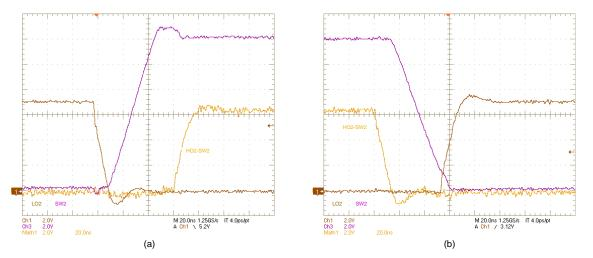
Figure 36. SW2, LO2, (HO2–SW2) Voltages:  $V_{IN}$  = 12 V,  $V_{OUT}$  = 12 V,  $I_{OUT}$  = 0 A, (a) OFF, (b) ON
