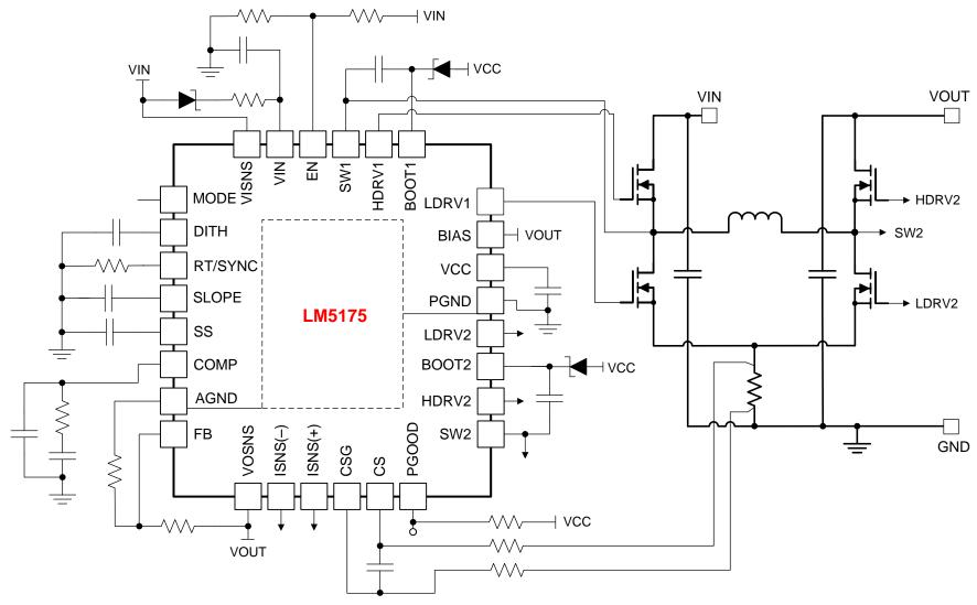
Figure 1. LM5175 Buck-boost Converter Circuit Diagram
