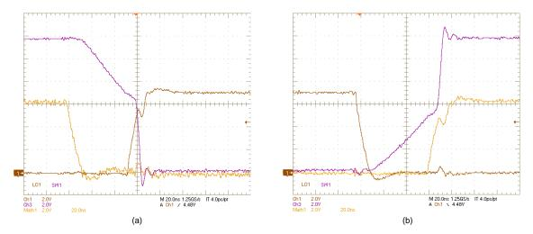
Figure 20. SW1, LO1, (HO1–SW1) Voltages:  $V_{IN} = 12 \text{ V}$ ,  $V_{OUT} = 12 \text{ V}$ ,  $I_{OUT} = 0 \text{ A}$ , (a) OFF, (b) ON
