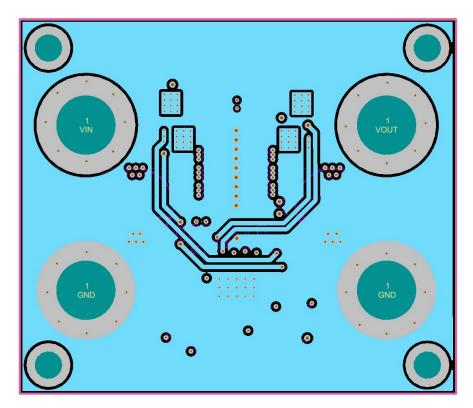
Figure 54. Layer 3 (Top view)
