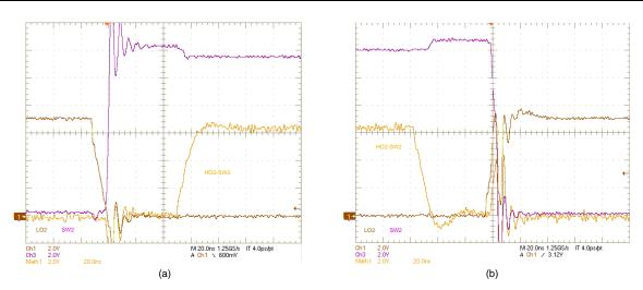
Figure 40. SW2, LO2, (HO2–SW2) Voltages:  $V_{IN}$  = 10 V,  $V_{OUT}$  = 12 V,  $I_{OUT}$  = 6 A, (a) OFF, (b) ON
