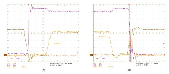
Figure 41. SW2, LO2, (HO2–SW2) Voltages:  $V_{IN}$  = 12 V,  $V_{OUT}$  = 12 V,  $I_{OUT}$  = 6 A, (a) OFF, (b) ON
