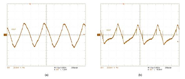
Figure 48.  $V_{OUT}$  ripple:  $V_{IN}$  = 24 V,  $V_{OUT}$  = 12 V, (a)  $I_{OUT}$  = 0 A, (b)  $I_{OUT}$  = 6 A
