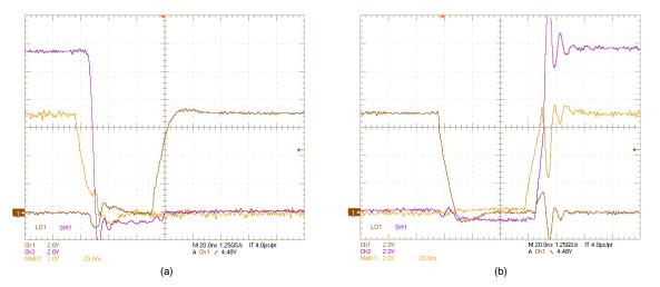
Figure 27. SW1, LO1, (HO1–SW1) Voltages:  $V_{IN}$  = 12 V,  $V_{OUT}$  = 12 V,  $I_{OUT}$  = 6 A, (a) OFF, (b) ON
