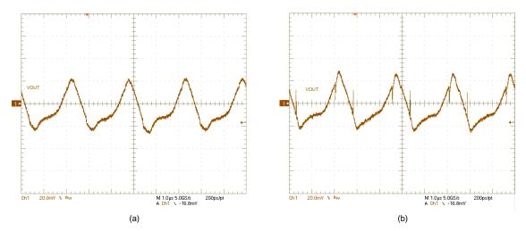
Figure 47.  $V_{OUT}$  ripple:  $V_{IN}$  = 18 V,  $V_{OUT}$  = 12 V, (a)  $I_{OUT}$  = 0 A, (b)  $I_{OUT}$  = 6 A
