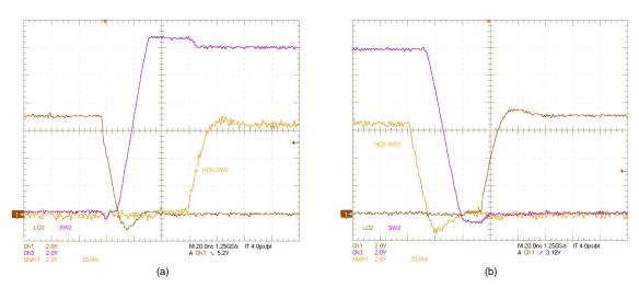
Figure 34. SW2, LO2, (HO2–SW2) Voltages:  $V_{IN} = 8 \text{ V}$ ,  $V_{OUT} = 12 \text{ V}$ ,  $I_{OUT} = 0 \text{ A}$ , (a) OFF, (b) ON
