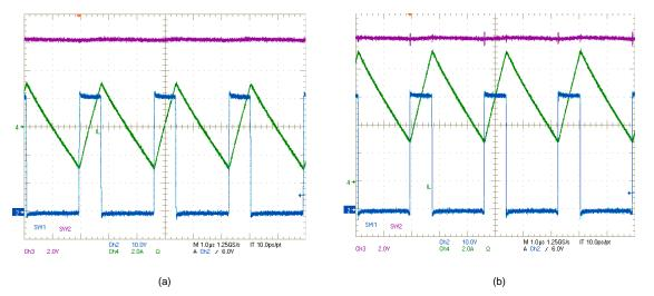
Figure 18. SW1, SW2,  $I_L$  Waveforms:  $V_{IN}$  = 42 V,  $V_{OUT}$  = 12 V, (a)  $I_{OUT}$  = 0 A, (b)  $I_{OUT}$  = 6 A
