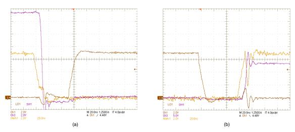
Figure 28. SW1, LO1, (HO1–SW1) Voltages:  $V_{IN} = 14 \text{ V}$ ,  $V_{OUT} = 12 \text{ V}$ ,  $I_{OUT} = 6 \text{ A}$ , (a) OFF, (b) ON
