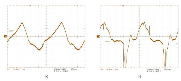
Figure 46.  $V_{OUT}$  ripple:  $V_{IN}$  = 14 V,  $V_{OUT}$  = 12 V, (a)  $I_{OUT}$  = 0 A, (b)  $I_{OUT}$  = 6 A
