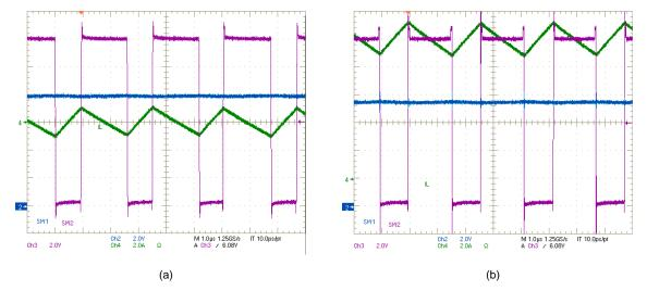
Figure 10. SW1, SW2,  $I_L$  Waveforms:  $V_{IN}$  = 8 V,  $V_{OUT}$  = 12 V, (a)  $I_{OUT}$  = 0 A, (b)  $I_{OUT}$  = 6 A
