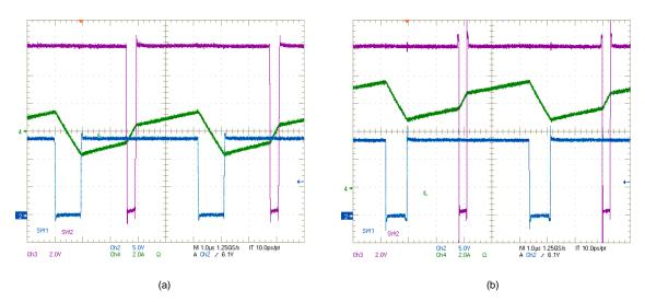
Figure 13. SW1, SW2,  $I_L$  Waveforms:  $V_{IN}$  = 14 V,  $V_{OUT}$  = 12 V, (a)  $I_{OUT}$  = 0 A, (b)  $I_{OUT}$  = 6 A
