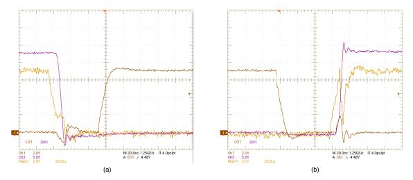
Figure 30. SW1, LO1, (HO1–SW1) Voltages:  $V_{IN}$  = 24 V,  $V_{OUT}$  = 12 V,  $I_{OUT}$  = 6 A, (a) OFF, (b) ON
