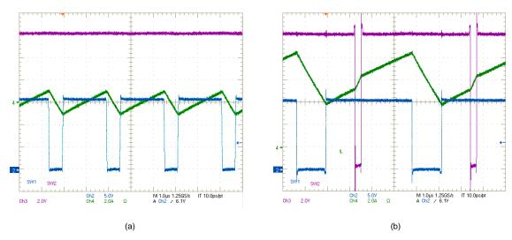
Figure 14. SW1, SW2,  $I_L$  Waveforms:  $V_{IN} = 16$  V,  $V_{OUT} = 12$  V, (a)  $I_{OUT} = 0$  A, (b)  $I_{OUT} = 6$  A
