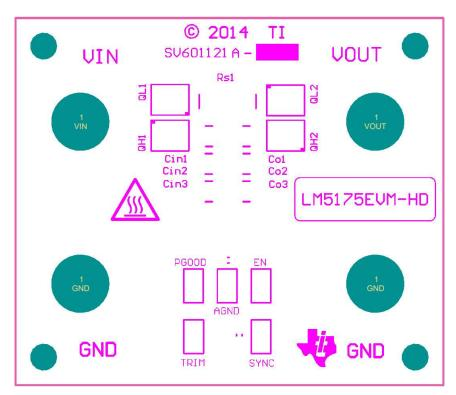
Figure 58. Top Layer Silkscreen (Top view)
