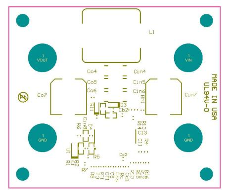
Figure 59. Bottom Layer Silkscreen (Bottom view)
