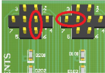
**Figure 1. Backlight LED Configuration Example**
