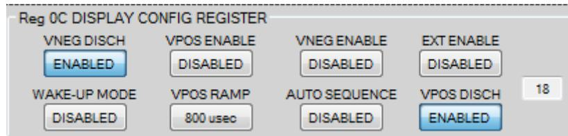
Figure 12. Display Bias Configuration Register Fields
