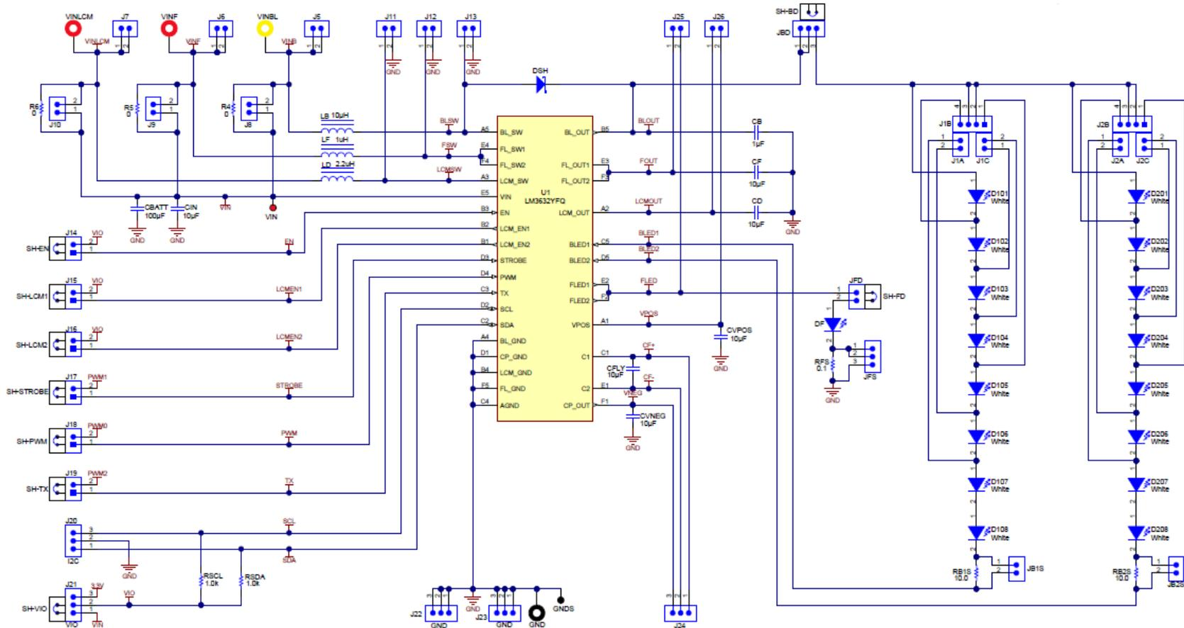
Figure 9. LM3632EVM Schematic
