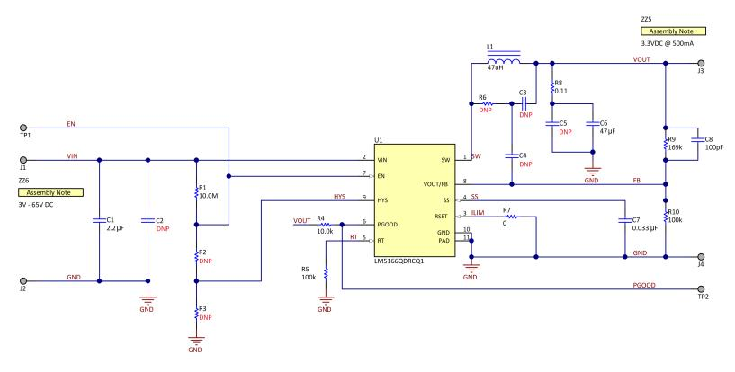
Figure 52. 3.3V, 500mA COT Schematic (Adjustable Output Version)
