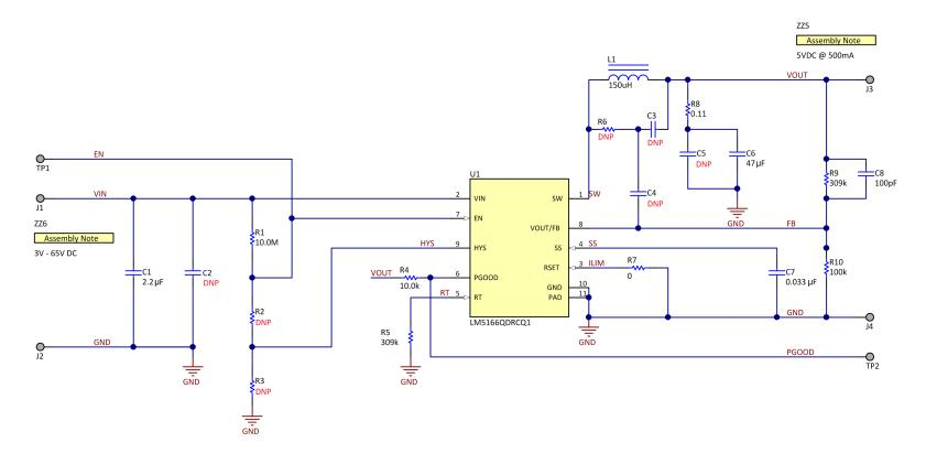
Figure 45. 5V, 500mA COT Schematic (Adjustable Output Version)
