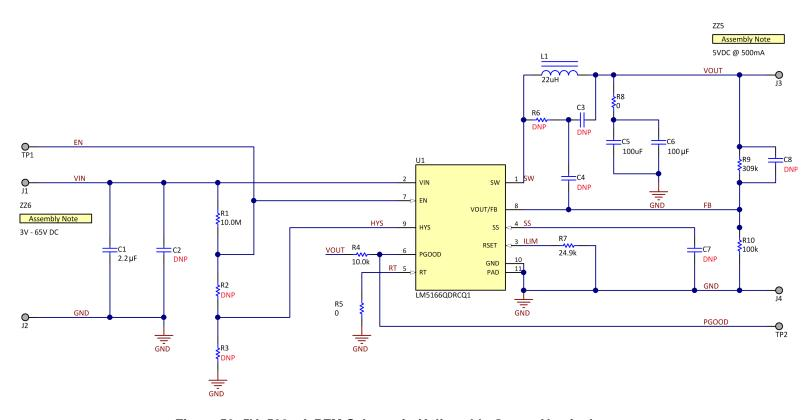
Figure 53. 5V, 500mA PFM Schematic (Adjustable Output Version)
