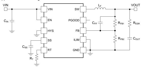
Figure 1. LM5166 Buck Converter Default Schematic: Adjustable Output COT
