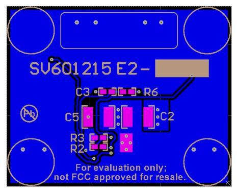
Figure 49. Bottom Copper (Bottom View)
