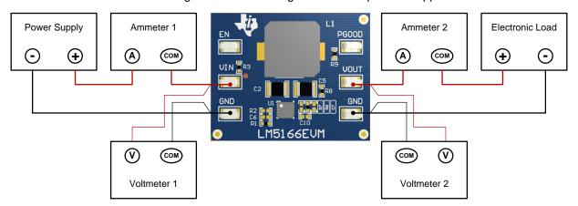
Figure 3. EVM Test Setup
