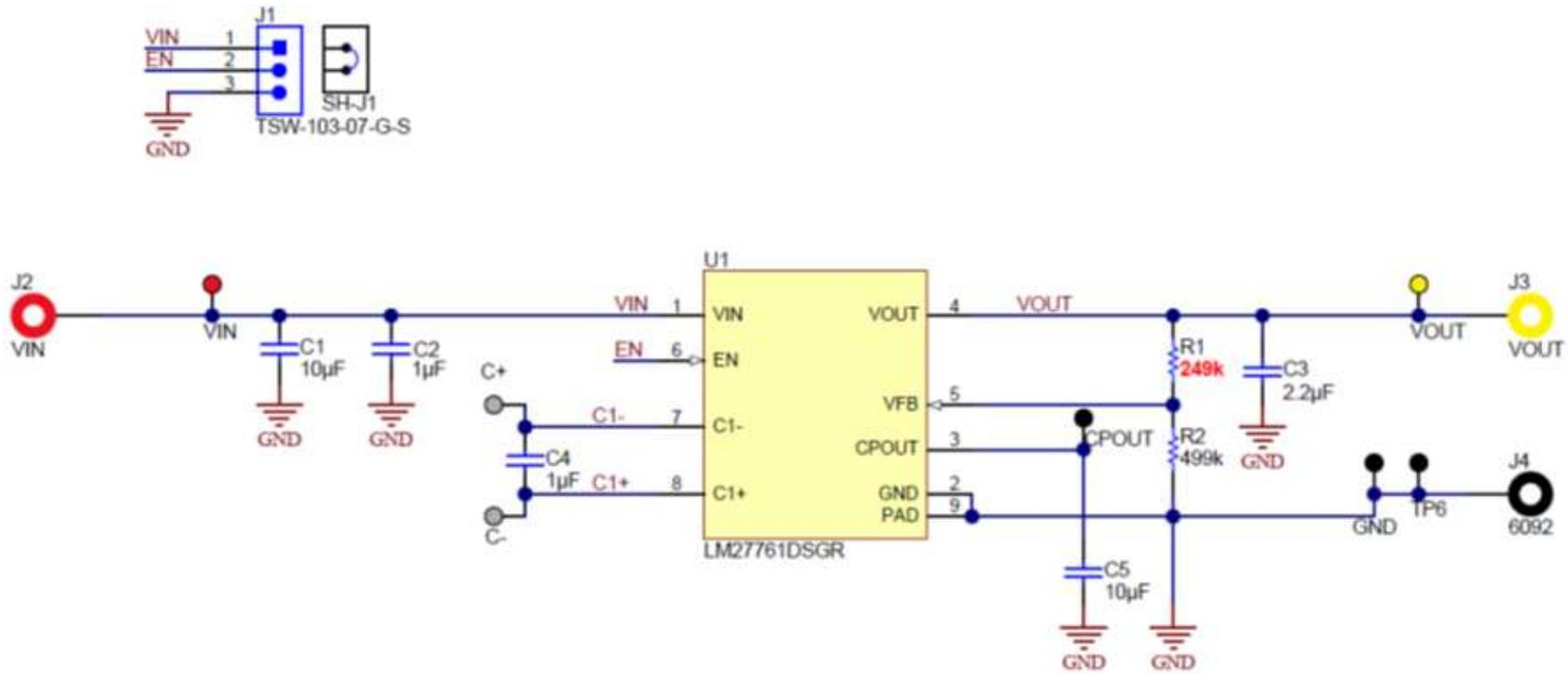
Figure 4. LM27761EVM Schematic
