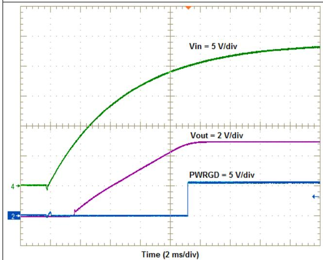
Figure 6. LMZ34202EVM Start-up Waveforms
