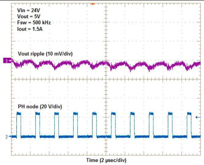
Figure 5. LMZ34202EVM Ripple Voltage (Fsw = 500 KHz)
