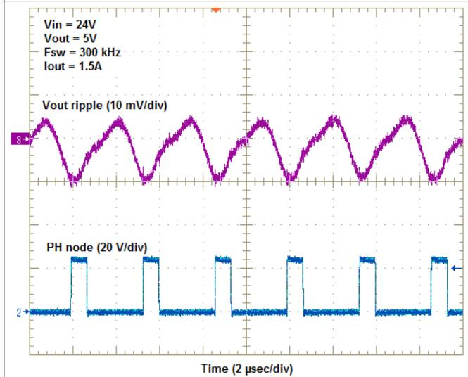
Figure 4. LMZ34202EVM Ripple Voltage (Fsw = 300 KHz)
