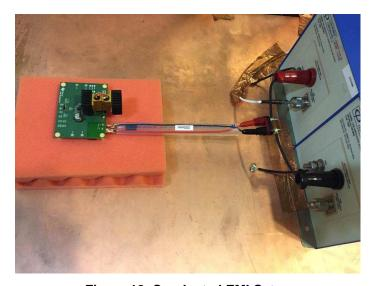
Figure 18. Conducted EMI Setup
