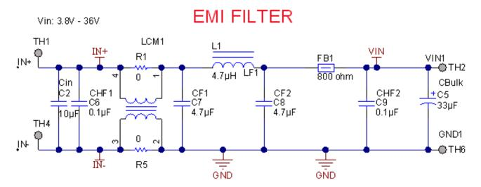
when laying out the board, keep the EMI filter away from Switch Node.
