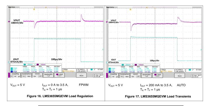
**NOTE:** The output capacitance for all four variants is designed for stable operation across all load transients and optimized performance with a maximum load transient of 0 to 3.5 A. For applications which require superior load transient performance beyond this range, TI recommends increasing the output capacitance. The best starting point for an optimized design is the Texas Instruments WEBENCH Design Tool.
