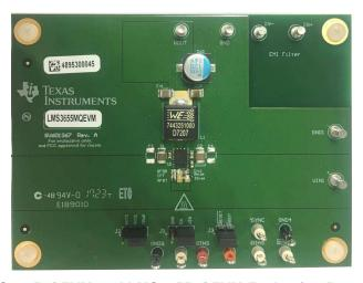
Figure 1. LMS3635xQEVM and LMS3655xQEVM Evaluation Board – Top View
