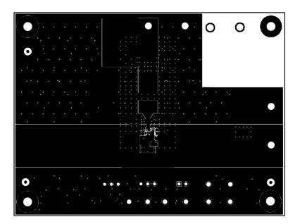
Figure 5. PCB Layout Top Layer 1 – Top View
