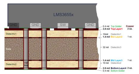
Figure 4. Four-Layer PCB Stack-Up
