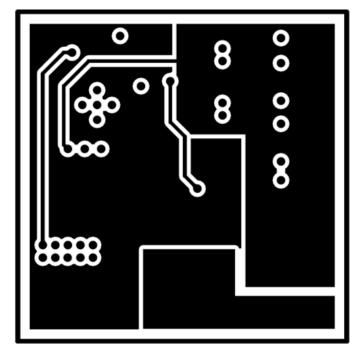
Figure 11. Mid2 Copper (X-Ray View)
