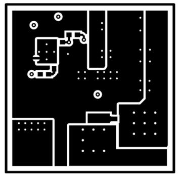
Figure 12. Bottom Copper (X-Ray View)
