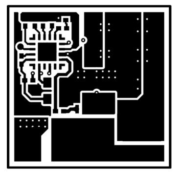
Figure 9. Top Copper (Top View)
