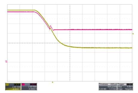
Figure 4. Cold-Cranking Using Cranking Simulator(C1:V<sub>SUPPLY</sub>, C2:V<sub>LOAD</sub>)
