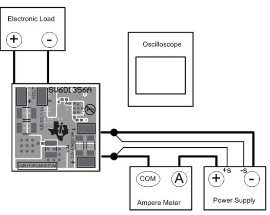
Figure 1. Standard Connection Diagram
