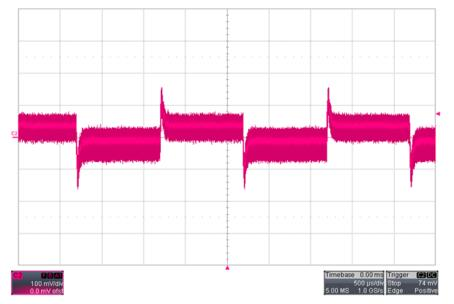
Figure 5. Load Transient(C2: V<sub>LOAD</sub> AC-coupled)
