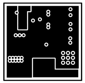
Figure 10. Mid1 Copper (X-Ray View)
