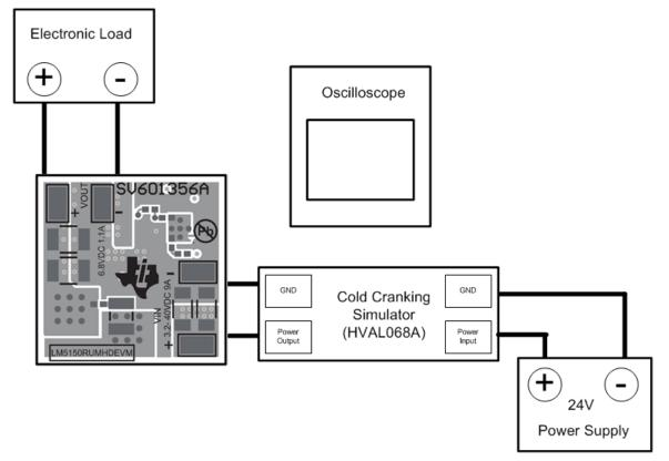
Figure 2. Cranking Simulator Connection Diagram
