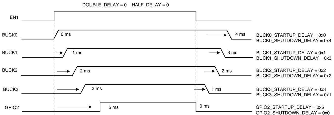
Figure 4. Startup and Shutdown Sequence Timing Diagram
