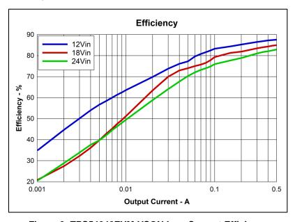
Figure 3. TPS54240EVM-VSON Low Current Efficiency
