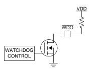
Figure 10. Open-Drain WDO Configuration
