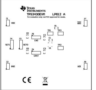
Figure 3. Component Placement—Top Overlay
