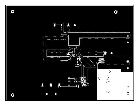
Figure 7. Top Layer Routing
