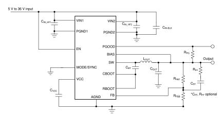
Figure 2. LM62440-Q1 Application Circuit
