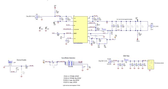
Figure 5. LM62440EVM-PP-2MHz Schematic
