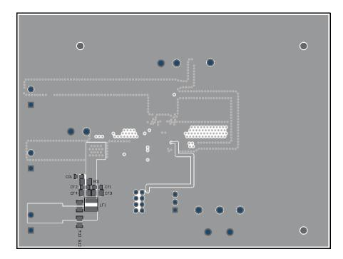
Figure 11. Bottom Component Layer and Silkscreen
