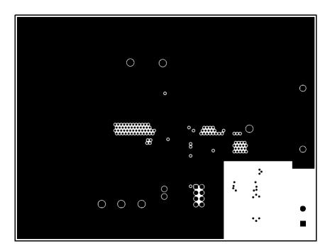
Figure 8. Mid-layer 1 Routing
