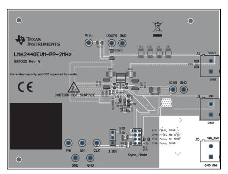
Figure 3. Top Component View of LM62440EVM-PP-2MHz
