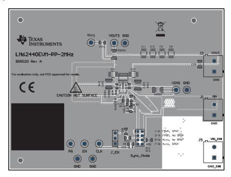
Figure 6. Top Component Layer and Silkscreen
