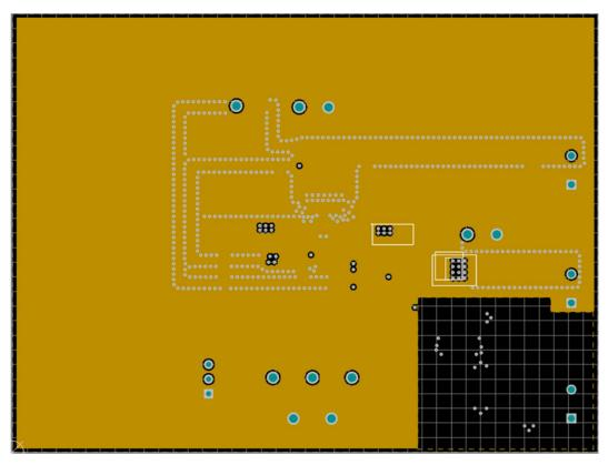
Figure 5-3. Signal Layer 1 - Ground Plane
