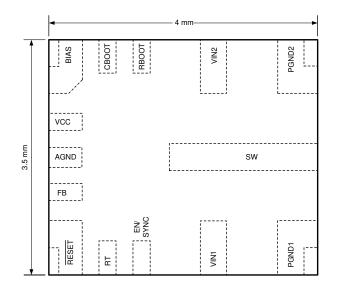
Figure 1-1. LMQ61460-Q1 Pin Configuration (Top View)
