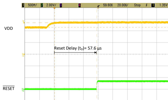
Figure 16. TLV840EVM \overline{\text{RESET}} Delay Time ( t_D ) with C_T Floating
